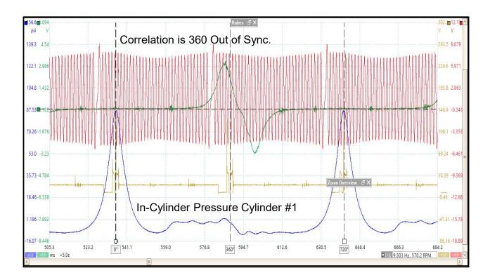
An In-Cylinder Pressure Transducer was added to Cylinder #1 (blue trace). The above waveform shows the Camshaft Sensor signal is 360 degrees "Out of Time". When the technician installed the synchronizer, Cylinder #1 was at Top Dead Center Exhaust (meaning Cylinder #5 was at Top Dead Center Compression).
