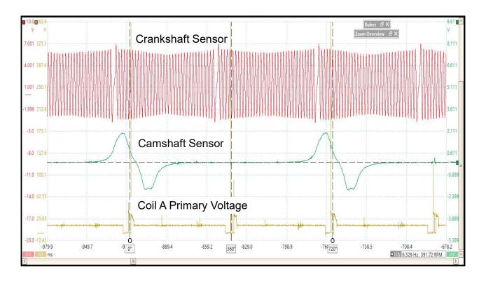
This particular engine uses a 36 – 1 Tooth Crankshaft Reluctor (35 pulses, each representing 10 degrees of crankshaft rotation). The two wire permanent magnet type sensor creates an A/C Sine Wave and missing tooth on Ford's V6 engines represents 60 degrees before Top Dead Center Compression Cylinder #1 and Cylinder #5 (meaning in two revolutions of the crankshaft the anomaly will show itself twice).
