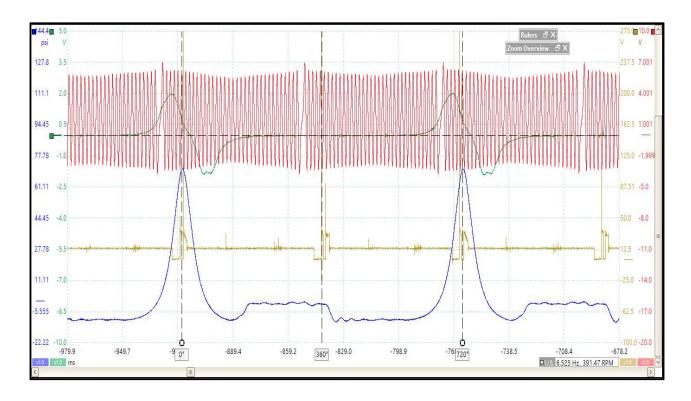
Now the Synchronizer has been moved to its correct position 26 Degrees After Top Dead Center Compression Cylinder #1.
