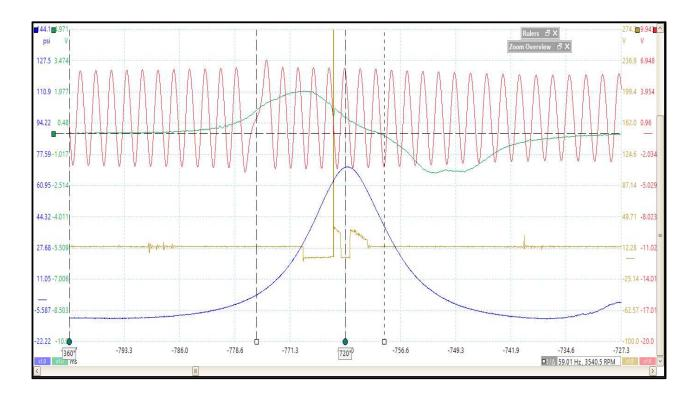
To confirm its correct position a zoomed image was taken to confirm its correlation. The Camshaft Sensor transitions from high (+ voltage) to low (- voltage) at 26 Degrees After Top Dead Center Compression.
