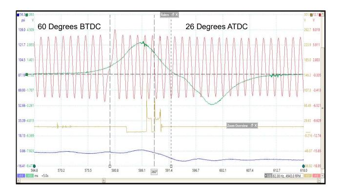
Zooming into the waveform the Crankshaft / Camshaft Correlation can be measured. Because with Ford we know the missing tooth represents 60 Degrees Before Top Dead Center we can count over 8 1/2 Teeth to check the correlation.
